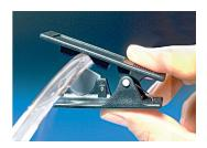
This handy pocket-sized tubing cutter will cut tubing from 1.5 mm to 13 mm outer diameter with a minimum of effort. Hardened steel blade produces clean right angle cuts. Cutter jaw is spring loaded and closes automatically. Blades are easily replaced and extra blades are sold separately. Does not cut rubber tubing.
